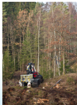
On a medium-sized forwarder, the Bracke M24.a provides very good scarification results on all mounding sites.
