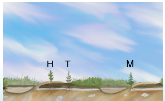
The Bracke M24.a creates planting spots with inverted humus (T), mineral soil mounds on inverted humus (H), and mineral soil mounds (M).
