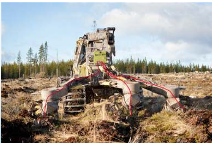
The Bracke S35.a can be attached to a one-, two-, or three-row scarifier.
