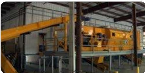
The CBI AirMax material separator component is versatile for C&D recycling, glass recycling, mulch cleanup, compost cleanup and automotive fluff recycling. The AirMax requires minimal power from four motors totaling 32 HP.
