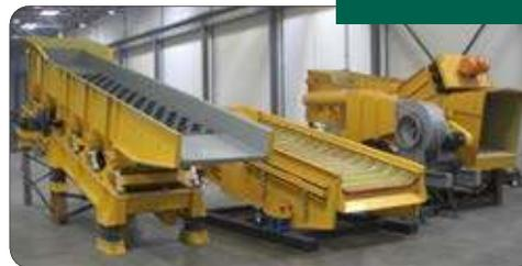
CBI offers a wide variety of screening solutions such as Taper Slot and Vibratory screens to meet the various needs of our customer and the wide range of materials they process.
