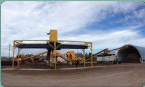
Continental Biomass Industries (CBI) recently designed and installed an electric stationary system that is customized to grind 600 - 800 tons of railroad ties on a daily basis. Ties 2, based out of northern Wisconsin, initially approached CBI about possible system options nearly two years ago and the planning process took off not long afterwards.
