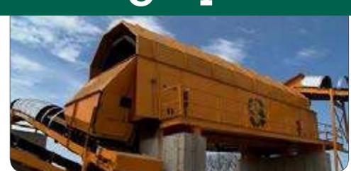
Trommel Screens effectively separate out fines from over-sized material. Ideal for applications requiring final product to be 2-inch and smaller.
